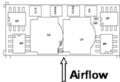
Figure 55. Airflow direction for thermal testing.
